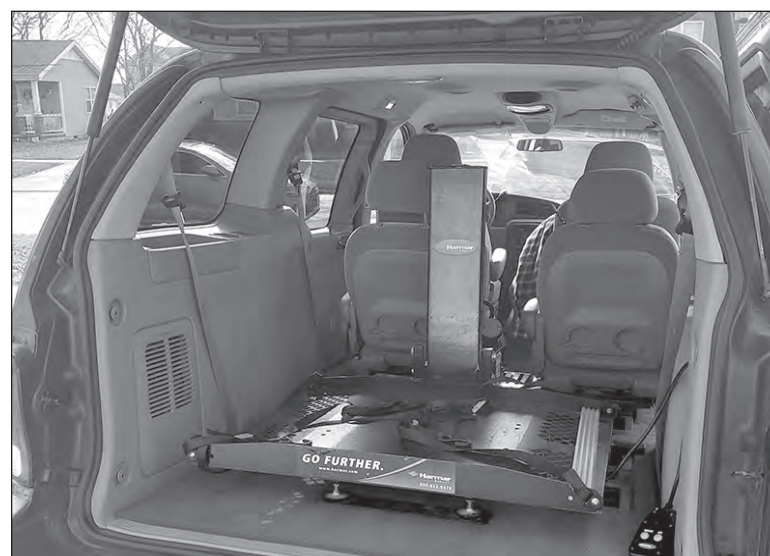
The handicap accessible vehicle is equipped with a lift chair assembly.
